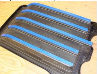
4. Turn the sled over and tighten the nylock nuts and larger washer onto the allen screw. The screws should hold in place while tightening them down if the correct size hole was drilled and they were not over tightened. Tighten until snug.
