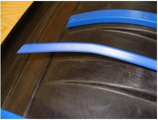
2. Center the strip on the rib, and using the hole in the hyfax strip as a guide, drill a hole into the sled using a 1/8" drill bit. Attach the strip to the sled using the provided allen screw and small washer. Using an allen bit and drill/driver will allow the screw to be driven into the small hole in the plastic. Turn in until just barely tight. This may be done by hand but will require more effort.
